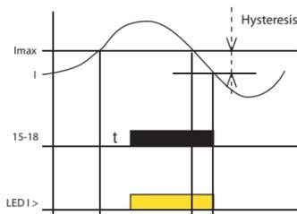
Monitoring relay PRI-52 serves for monitoring of current level in 1-phase AC circuits. Slight setting of release current level designates this relay for many various applications. Output relay is in normal status switched off. When set current level is overrun, relay get closed after preset delay. By return from error to normal status is used hysteresis.
