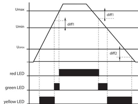
After connecting the supply voltage, the LED illuminates - the color corresponds to the voltage size of individual phases. If the phase voltage drops under 40 V (phase outage), the corresponding LED is not illuminated.
