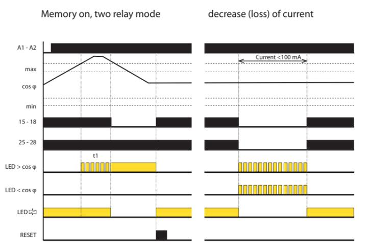
After powering on, the device sets the delay time t1 and yellow LED flashes. Both relays are switched on. The delay serves to eliminate a faulty state when starting the motor. After the time delay t1 begins monitoring COS φ only.
