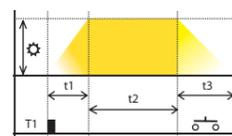
Dim-up delay-down is started by a button. Cycle extension - by re-pressing button (during the cycle).
