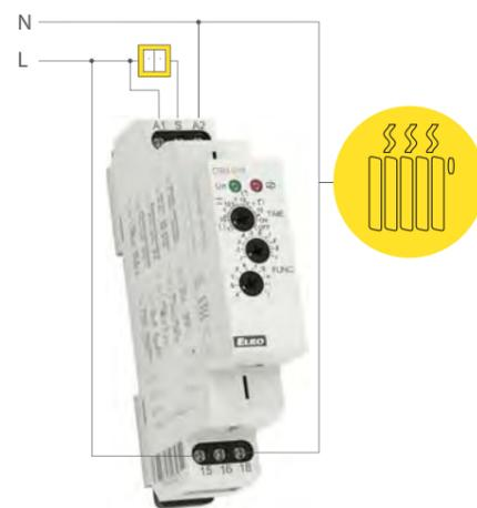
**Multifunction time relay with contactless output CRM-9S**
