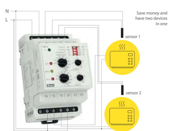
**Thermostat for thermal protection of motors TER-7**
