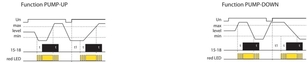
An AC current is used for measuring to prevent polarization and electrolysis of fluid and unwanted oxidation of measuring probes. Three probes are used for measuring: H - upper level, D - lower level and C - common probe. If using a tank made from conductive material, it is possible to use the tank itself as probe C.
