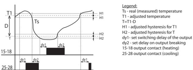
In case of thermostat with a „dead zone“, it is possible to set temperature T1 and a difference (respectively a width of dead zone D). If temperature is higher than T1, output contact of cooling switches ON; if the temperature gets below T1, the contact switches OFF.
