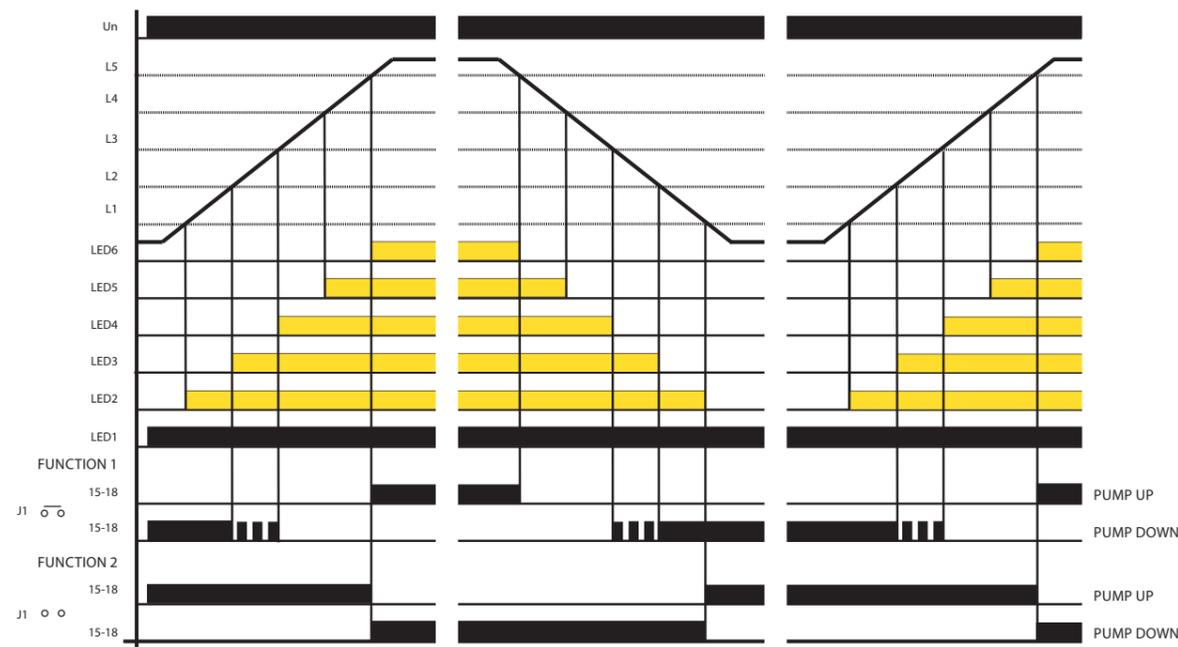
This device monitors level of a conductive liquid in a tank by using six single probes or one 6-fold probe. In case you use a tank made of a conductive material, it is possible to use it as a common probe C.
