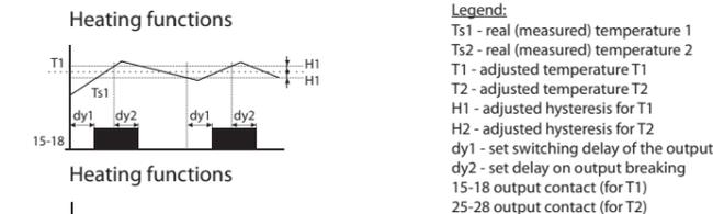
Classic function of thermostat, output contact switched until adjusted temperature is reached. Hysteresis eliminates frequent switching - output oscillation.
