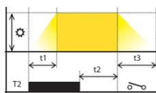
The switch starts the cycle and it stops on max.set brightness. After the switch is off, the cycle will continue until completed.
