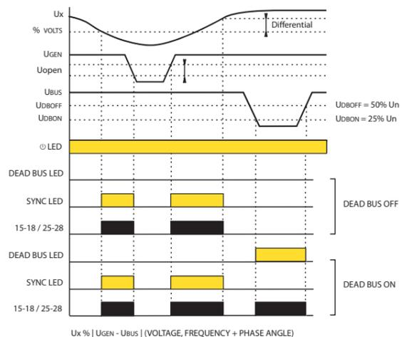
The differential trip levels help to prevent relay chatter as the monitored voltage level varies.
