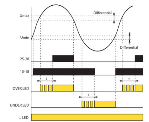
The time delay and differential trip levels help to prevent relay chatter as the monitored voltage level varies. As the relays have changeover contacts, the relay outputs can be inverted by wiring to the alternative terminals 15-16 or 25-26.
