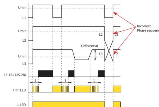
The time delay and differential trip levels help to prevent relay chatter as the monitored parameter fluctuates.
