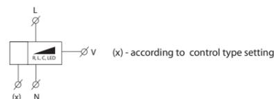
\* Warning: it is not allowed to connect inductive and capacitive loads at the same time.
