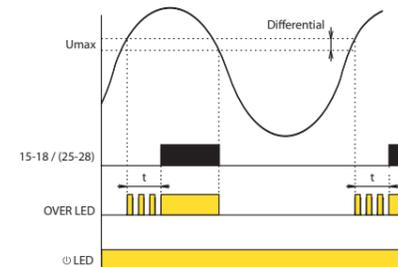
The time delay and differential trip levels help to prevent relay chatter as the monitored voltage level varies. As the relays have changeover contacts, the relay outputs can be inverted by wiring to the alternative terminals 15-16 or 25-26.
