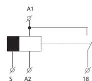
\* For bigger bulb loads and frequent switching is recommended to intensify the contact relay with power contactor e.g. VSXXX
