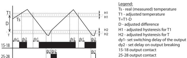
Typical example of use for two-stage thermostat is e.g. in boiler-room, where there are two boilers from which one is main and the other one is auxiliary. The main boiler is managed according to set temperature and auxiliary boiler is switched in case temperature falls under set difference. Thus it helps to the main boiler in case outside temperature dramatically falls.
