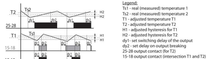
Output 15-18 is closed, if temperature of both thermostats is below an adjusted level. When any thermostat reaches adjusted level, the contact 15-18 opens. Serial inner connection of thermostats (logic function AND).
