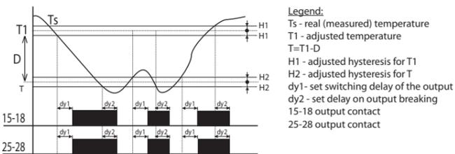
Output is closed (heating) only if temperature is within adjusted range. If temperature is out of range, the contact opens. T is set as T1-D.
