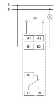
**Example Connection:** PRI-51 with current transformer for current range increase.
