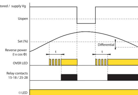
The time delay and differential trip levels help to prevent relay chatter as the monitored parameters fluctuate.
