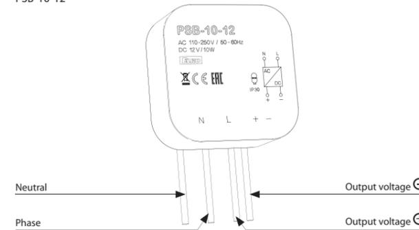
PSB-10-12 / PSB-10-24 designated for installation into an installation box. Suitable for controlling of lighting sources, thermo valves, shutter engines, etc.
