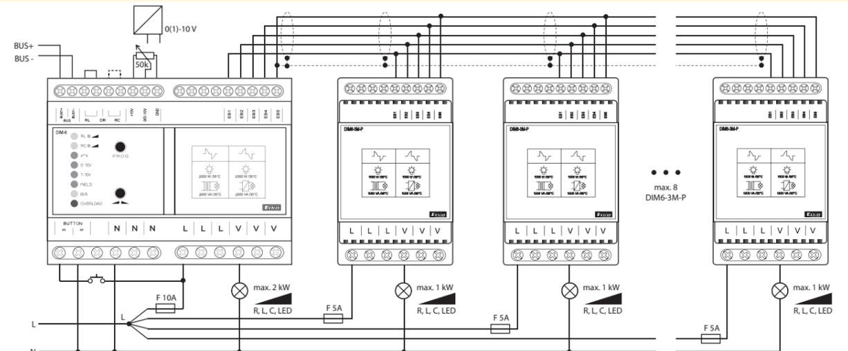
A quick fuse corresponding to the power of each module must be included in the L supply for each module.
