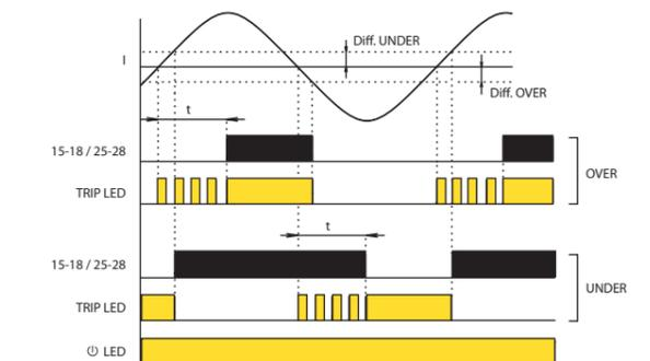
After the supply voltage is connected the green LED is on.
