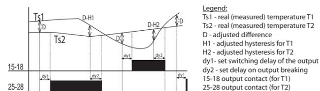
Switching of output corresponds with input, which has lower temperatures when difference is exceeded.
