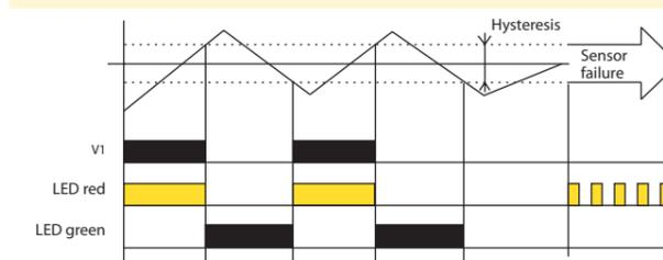
TEV-2 and TEV-3 are universal single thermostats for universal use. In case ambient temperature is higher than set temperature relay is open (function HEATING), for cooling function (opposite function) is possible to use NC contact of relay (V2).
