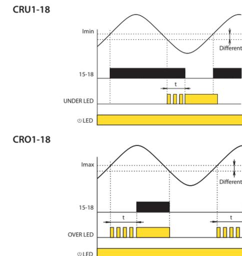
The time delay and differential trip levels help to prevent relay chatter as the monitored current level varies. As the relays have changeover contacts, the relay outputs can be inverted by wiring to the alternative terminals 15-16 or 25-26.
