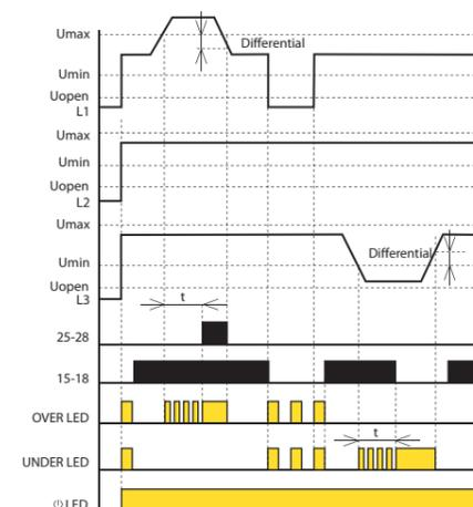
The time delay and differential trip levels help to prevent relay chatter as the monitored voltage level varies.
