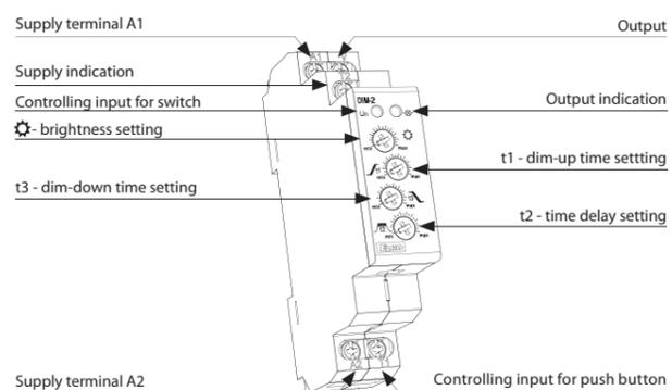
Recommendation for mounting: leave a gap of min. 0.5 module (approx. 9 mm) on side of the device to ensure better cooling of the device.
