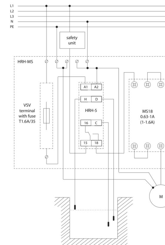
**Level set HRH-MS-VS-2.5A (HRH-MS-VS-4A, HRH-MS-VS-6.3A)**
