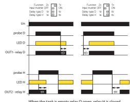
When the tank is empty relay D open, relay H is closed.
