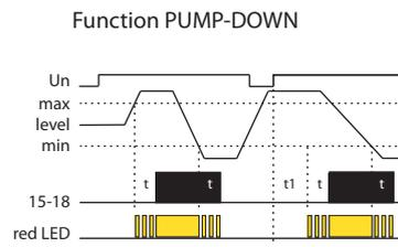
An AC current is used for measuring to prevent polarization and electrolysis of fluid and unwanted oxidation of measuring probes. Three probes are used for measuring: H - upper level, D - lower level and C - common probe. If using a tank made from conductive material, it is possible to use the tank itself as probe C.
