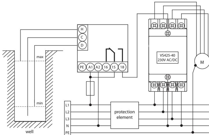
Monitoring TWO LEVELS minimum/maximum - DRAINING function - (PUMP DOWN)
