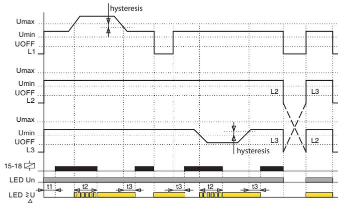
The relay in a 3-phase network monitors the phase voltages magnitude. Two independent voltage levels can be set to monitor undervoltage and overvoltage separately.
