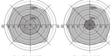
ceiling installation height: 2.5m detecting range setting:100%/50% ceiling installation height: 3m detecting range setting:100%/50% 10
