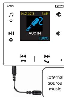
The input **AUX IN** is used to connect external audio devices such as a mobile phone, mp3 player and others. A 3.5 mm jack provides connection. In this mode, the player functions as an audio amplifier. When activating the input, the volume on the player is set (fixed) at 100%. You can control only on a connected external audio device.
