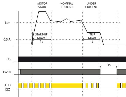
Right after connecting a supply voltage, an output relay is immediately closed and waits for a motor to be started by a START button. Once the START button is activated a contactor closes and the motor starts. An auxiliary contact of the contactor bridges the START button and keeps the contactor closed.
