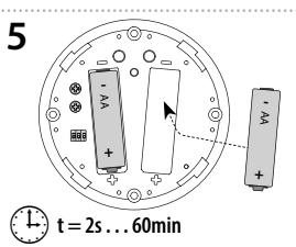
After setting the desired time (within 2s ... 60 min), the timer mode ends by inserting the battery into the detector. The red LED on the detector will blink. This saves the time interval stored in the memory of the component, the LED on the compatible component blinks.
