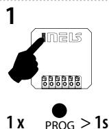
Press of programming button on compatible actuator for 1 second will activate actuator into programming mode. LED is flashing in 1s interval.
