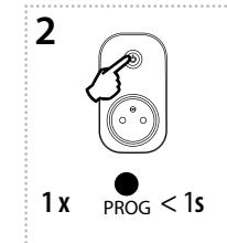
By one short press of the programming button on the RFRP-20N, you move to the position for input into the additional learning mode. The red LED flashes - after 5s the RFRP-20N enters the additional learning mode. The LED stops flashing.
