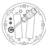
Set the DIP switch (e.g. with a screwdriver).
