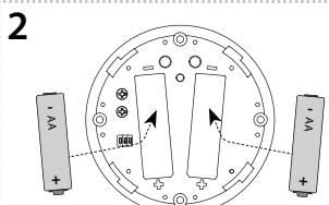
Slide the battery into the battery holder in the detector. Beware of polarity. The red LED on the detector will blink. The LED on a compatible component will blink at a faster interval - thereby assigning the detector to the component.
