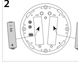
Slide the battery into the battery holder in the detector. Beware of polarity. The red LED on the detector will blink. The LED on a compatible component will blink at a faster interval - thereby assigning the detector to the component.
