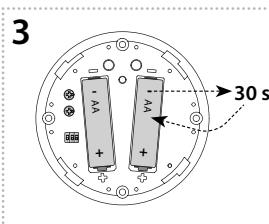
Remove one of the batteries from the detector and insert it back after 30 seconds. The red LED on the detector will blink. The LED on a compatible component will blink at a faster interval.
