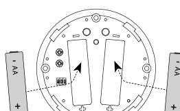
Insert the batteries into the battery holder in the detector. Beware of polarity. The red LED on the detector will blink - setting the DIP switch setting.
