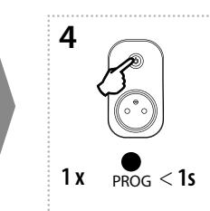
End learning mode by a short press of the programming button on the RFRP-20N. By doing so, the programmed address detector is stored in the memory. The red LED will flash for 1 second, then the green LED will remain illuminated.
