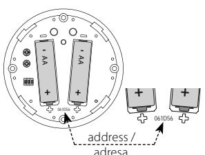
For the programming and communication of the detector with the system components, the address shown on the underside of the detector or in the left upper part of the open device is used.
