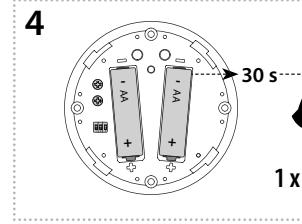
Remove the battery from the detector again. After 30 seconds, press the programming button for more than 5 seconds to bring the compatible component into timer mode. LED 2x blinks at second intervals. When the button is released, delayed return time is retrieved.
