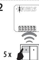
Assignment of the sunrise function is performed by five presses of the selected button on the RF transmitter (must be a lapse of 1s between individual presses).
