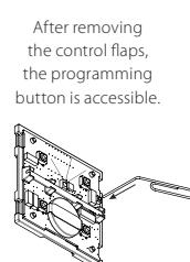
After removing the control flaps, the programming button is accessible.
