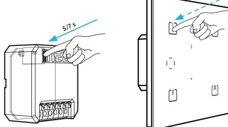
To clear an already paired channel to a button on the controller, press the PROG on the device for a period of time of 5 s or 7 s (see. Tab 1). Clear the memory of the button and press the appropriate button on the controller that you want to unpair. After this step, the item returns to its working state.
