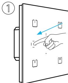
Press of programming button on receiver RFDW-71 for 1 second will activate receiver into programming mode. LED is flashing in 1s interval.
