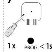
Press of programming button on receiver RFJA shoter then 1 second will finish programming mode (LED switches off).
