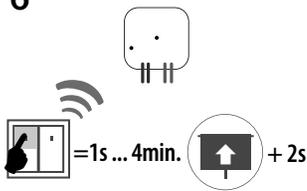
Press of the button on wireless switch with assigned function for shutters up will roll the shutters up. Release the press of this button 2 seconds after the shutter is stopped by upper final switch. Duration of rolling up and down is than saved into memory of receiver.
