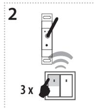
Three presses of your selected button on the RF transmitter assigns the function switch off (must be a lapse of 1s between individual presses).
