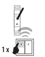
After the desired time has elapsed (range of 2s...60min), the timing mode ends by pressing the button on the RF transmitter, to which the delayed return function is assigned. This stores the set time interval into the actuator memory.
