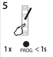
Press of programming button on receiver RFSA-61M/MI (66M/MI) shorter than 1 second will finish programming mode. The LED lights up according to the pre-set memory function.
