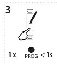
Press of programming button on receiver RFSA-61M/MI (66M/MI) shorter than 1 second will finish programming mode. The LED lights up according to the pre-set memory function.
