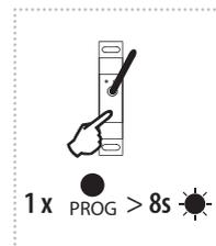
By pressing the programming button on the actuator for 8 seconds, deletion occurs of the actuator's entire memory. LED flashes 4x in each 1s interval.
