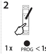
Pressing the programming button on the RFSA-61M/MI (66M/MI) receiver for less than 1 second will finish the programming mode, this will reverse the memory function. The LED lights up according to the current pre-set memory function. The set memory function is saved. Every other change is made in the same way.
