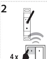
Four presses of your selected button on the RF transmitter assigns the function impulse relay (must be a lapse of 1s between individual presses).
