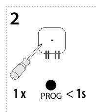
Pressing the programming button on the RFSAI-61B receiver for less than 1 second will finish the programming mode, this will reverse the memory function. The LED lights up according to the current pre-set memory function. The set memory function is saved.
