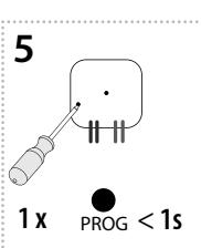
Press of programming button on receiver RFSAI-61B shorter than 1 second will finish programming mode. The LED lights up according to the pre-set memory function.
