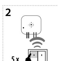
Assignment of the delayed off function is performed by five presses of the selected button on the RF transmitter (must be a lapse of 1s between individual presses).
