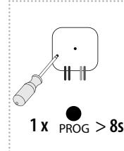
By pressing the programming button on the actuator for 8 seconds, deletion occurs of the actuator's entire memory. LED flashes 4x in each 1s interval. The actuator goes into the programming mode, the LED flashes in 0.5s intervals (max. 4 min.). You can return to the operating mode by pressing the Prog button for less than 1s. The LED lights up according to the pre-set memory function and the component returns to the operating mode. Deletion does not affect the pre-set memory function.
