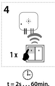
After the desired time has elapsed (range of 2s...60min), the timing mode ends by pressing the button on the RF transmitter, to which the delayed return function is assigned. This stores the set time interval into the actuator memory.
