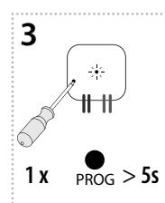
Press of programming button longer than 5 seconds, will activate actuator into timing mode. LED flashes 2x in each 1s interval. Upon releasing the button, the delayed return time starts counting.
