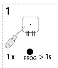
Press of programming button on receiver RFSAI-61B for 1 second will activate receiver RFSAI-61B into programming mode. LED is flashing in 1s interval.
