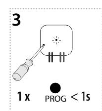
Press of programming button on receiver RFSAI-61B shorter than 1 second will finish programming mode. The LED lights up according to the pre-set memory function.
