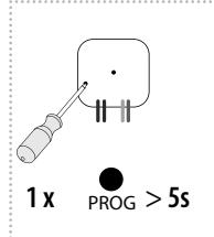
By pressing the programming button on the actuator for 5 seconds, deletion of one transmitter activates. LED flashes 4x in each 1s interval. Pressing the required button on the transmitter deletes it from the actuator's memory. To confirm deletion, the LED will confirm with a flash long and the component returns to the operating mode. The memory status is not indicated. Deletion does not affect the pre-set memory function.
