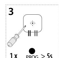
Press of programming button longer than 5 seconds, will activate actuator into timing mode. LED flashes 2x in each 1s interval. Upon releasing the button, the delayed return time starts counting.
