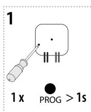
Press of programming button on receiver RFSAI-61B for 1 second will activate receiver RFSAI-61B into programming mode. LED is flashing in 1s interval.
