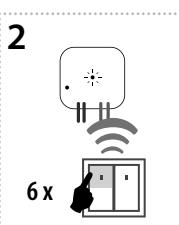
Assignment of the delayed on function is performed by six presses of the selected button on the RF transmitter (must be a lapse of 1s between individual presses).
