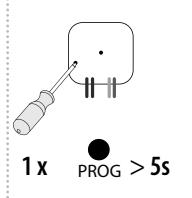
By pressing the programming button on the actuator for 5 seconds, deletion of one transmitter activates. LED flashes 4x in each 1s interval.
