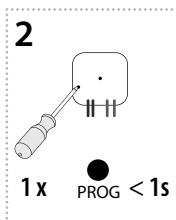
Pressing the programming button on the RFSAI-61B receiver for less than 1 second will finish the programming mode, this will reverse the memory function. The LED lights up according to the current pre-set memory function. The set memory function is saved.
