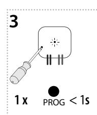
Press of programming button on receiver RFSAI-61B shorter than 1 second will finish programming mode. The LED lights up according to the pre-set memory function.
