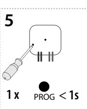
Press of programming button on receiver RFSAI-61B shorter than 1 second will finish programming mode. The LED lights up according to the pre-set memory function.
