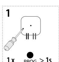
Press of programming button on receiver RFSAI-61B for 1 second will activate receiver RFSAI-61B into programming mode. LED is flashing in 1s interval.
