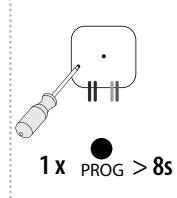
By pressing the programming button on the actuator for 8 seconds, deletion occurs of the actuator's entire memory. LED flashes 4x in each 1s interval.
