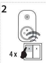
Four presses of your selected button on the RF transmitter assigns the function impulse relay (must be a lapse of 1s between individual presses).
