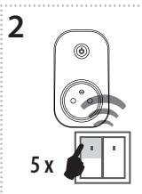
Assignment of the delayed off function is performed by five presses of the selected button on the RF transmitter (must be a lapse of 1s between individual presses).
