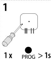
Press of programming button on receiver RFSA-x1B for 1 second will activate receiver RFSA-x1B into programming mode. LED is flashing in 1s interval.
