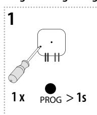
Press of programming button on actuator RFSA-11B for 1 second will activate actuator RFSA-11B into programming mode. LED is flashing in 1s interval.
