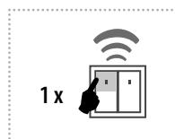
The output contact will be closed by pressing the button and opened after the set time interval has elapsed.
