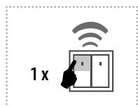
The output contact will be closed by pressing the button and opened by releasing the button.
