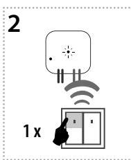
Select and press one button on wireless switch, to this button will be assigned function Button.
