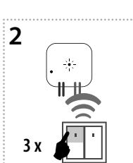
Three presses of your selected button on the RF transmitter assigns the function switch off (must be a lapse of 1 s between individual presses).
