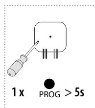
By pressing the programming button on the actuator for 5 seconds, deletion of one transmitter activates. LED flashes 4x in each 1s interval. Pressing the required button on the transmitter deletes it from the actuator's memory. To confirm deletion, the LED will confirm with a flash long and the component returns to the operating mode. The memory status is not indicated. Deletion does not affect the pre-set memory function.
