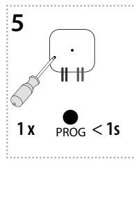
Press of programming button on actuator RFSA-61B shorter than 1 second will finish programming mode. The LED lights up according to the pre-set memory function.
