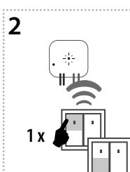
Pressing your chosen button on the RF transmitter assigns the function "close". The second position of the control "switch off" is assigned automatically (for 4-button in the same half of the RF transmitter).
