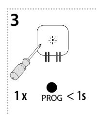
Press of programming button on actuator RFSA-61B shorter than 1 second will finish programming mode. The LED lights up according to the pre-set memory function.
