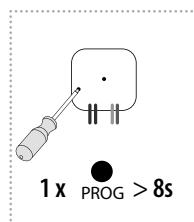
By pressing the programming button on the actuator for 8 seconds, deletion occurs of the actuator's entire memory. LED flashes 4x in each 0.5s interval. The actuator goes into the programming mode, the LED flashes in 0.5s intervals (max. 4 min.). You can return to the operating mode by pressing the Prog button for less than 1s. The LED lights up according to the pre-set memory function and the component returns to the operating mode. Deletion does not affect the pre-set memory function.
