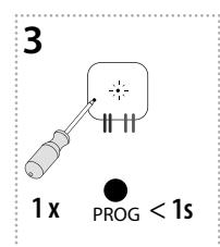
Press of programming button on actuator RFSA-11B shorter than 1 second will finish programming mode. The LED lights up according to the pre-set memory function.
