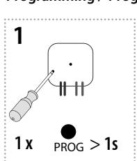
Press of programming button on actuator RFSA-61B for 1 second will activate actuator RFSA-61B into programming mode. LED is flashing in 1s interval.
