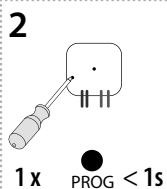
Pressing the programming button on the RFSA-x1B receiver for less than 1 second will finish the programming mode, this will reverse the memory function. The LED lights up according to the current pre-set memory function. The set memory function is saved.
