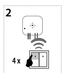
Four presses of your selected button on the RF transmitter assigns the function impulse relay (must be a lapse of 1 s between individual presses).
