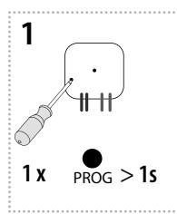
Press of programming button on actuator RFSA-61B for 1 second will activate actuator RFSA-61B into programming mode. LED is flashing in 1s interval.
