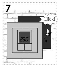
By pressing gently, seat the device into the lower part so that the holders of the lower part go through the broken out moldings in the frame.
