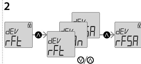
Unlock RFTC-10/G for modification by pressing **Ⓐ**. Set **DEV - rFSR** by pressing **Ⓐ**. Confirm settings by pressing **Ⓐ**.
