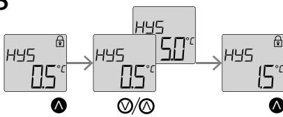
By pressing **Ⓐ**, you will move in Menu to **HYS** - switching hysteresis. Unlock the modifications menu by pressing **Ⓐ**. By pressing **V/O**, set the hysteresis based on individual requirement in the range of 0.5...5°C (1...10°F). Press **Ⓐ** to confirm settings.
