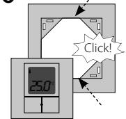
By pressing gently, snap the device into the frame.
