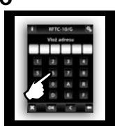
On the control unit, enter the address of RFTC-10/G (see manual of control unit).
