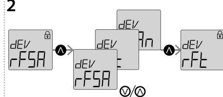
Unlock RFTC-10/G for modification by pressing  $\textcircled{A}$ . Set **DEV-RFT** by pressing  $\textcircled{A}$ . Confirm settings by pressing  $\textcircled{A}$ .
