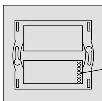
An address listed on the back of the actuator is used for programming and controlling the temperature actuator by RF Touch / eLAN-RF.
