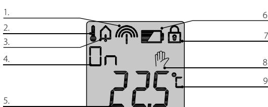
1. Signal strength - (1 bar - weak signal, 3 bars - strong signal) the symbol does not display if the controller is not programmed or it is not possible to establish a connection with the programmed switching unit or system unit.
