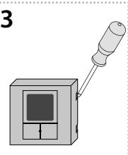
Using a screwdriver, gently slide the device out from the cover - be careful not to damage the device.
