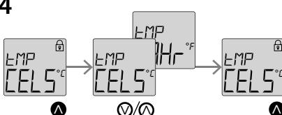
By pressing **Ⓐ**, you will move in Menu to **TEMP** - display of measured temperature value. Unlock the modifications menu by pressing **Ⓐ**. By pressing **V/O** select °C or °F. Press **Ⓐ** to confirm settings.
