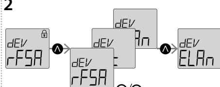
Unlock RFTC-10/G for modification by pressing **A**. Set **DEV - ELAN** by pressing **A**. Confirm settings by pressing **A**.
