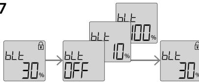
By pressing **Ⓐ**, you will move in Menu to **bLc** - display brightness (backlighting). Unlock the modifications menu by pressing **Ⓐ**. By pressing **V/O**, set the display brightness based on individual requirement in the range of 10% - 100%. Press **Ⓐ** to confirm settings.
