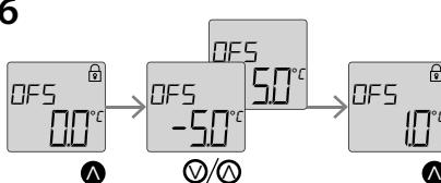
By pressing **Ⓐ**, you will move in Menu to **DFS** - offset of temperature sensor. By pressing **Ⓐ**, unlock the modifications menu. By pressing **V/O**, set the offset based on individual requirement in the range of -5...+5°C (-10...+10°F). Press **Ⓐ** to confirm settings.
