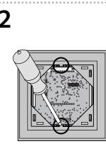
Using a screwdriver, carefully pry off the molding and snap out the device from the frame.
