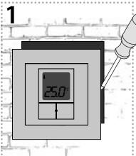
Using a screwdriver, remove the lower part.
