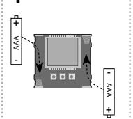
Remove the original dead batteries. Slide new batteries into the battery holder. Observe the polarity. After inserting the batteries, the FW version will appear for 1s, then the current measured temperature.
