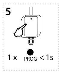
Press of programming button on receiver RFUS-61 shorter than 1 second will finish programming mode. The LED lights up according to the pre-set memory function.
