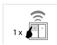
The output contact will be closed by pressing the button and opened by releasing the button. For the correct execution of individual commands (press = closing / releasing the button = opening), the time delay between these commands must be a min of. 1s (press - delay 1s - release).
