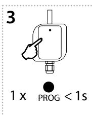
Press of programming button on receiver RFUS-61 shorter than 1 second will finish programming mode. The LED lights up according to the pre-set memory function.
