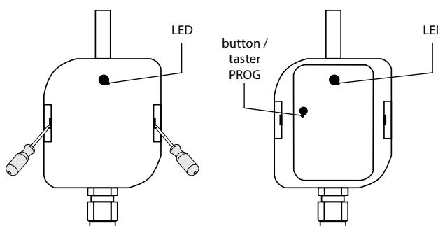
Before starting the programming / manual control, open the actuator housing using a screwdriver. After completing programming / manual control, snap the housing closed again.
