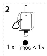
Pressing the programming button on the RFUS-61 receiver for less than 1 second will finish the programming mode, this will reverse the memory function. The LED lights up according to the current pre-set memory function. The set memory function is saved.
