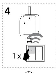
After the desired time has elapsed (range of 2s...60min), the timing mode ends by pressing the button on the RF transmitter, to which the delayed return function is assigned. This stores the set time interval into the actuator memory.
