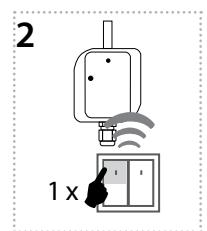
2 Select and press one button on wireless switch, to this button will be assigned function Button.
