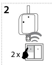
Two presses of your selected button on the RF transmitter assigns the function switch on (must be a lapse of 1s between individual presses).
