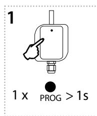
1 Press of programming button on receiver RFUS-61 for 1 second will activate receiver RFUS-61 into programming mode. LED is flashing in 1s interval.
